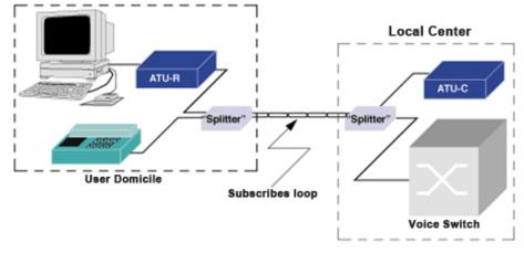
Since this is a modulation where different throughputs are transmitted in User -> Network and Network -> User directions, the ADSL modem at the user end (ATU-R or ADSL Terminal Unit-Remote) is different to the one at the other end of the loop (local central, ATU-C or ADSL Terminal Unit-Central).
