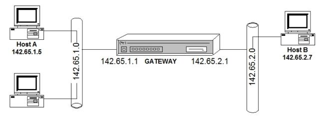
The *global* IP network corresponds to the 142.65.0.0 address with the 255.255.0.0 mask. It must be considered a Class B address.
