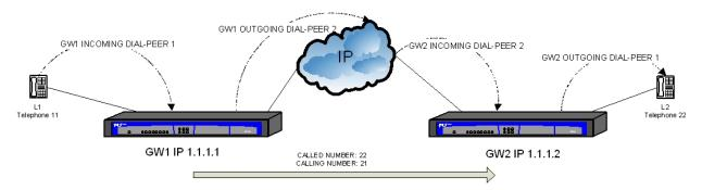
As shown in the diagram, for GW1, the call enters through dial-peer 1 as this dial-peer has router line 1 as its target. Once connected, the incoming dial-peer searches for the outgoing dial-peer and finds 2, as this has pattern 2., which matches called number 22, and forwards the call to IP 1.1.1.2 through SIP.
