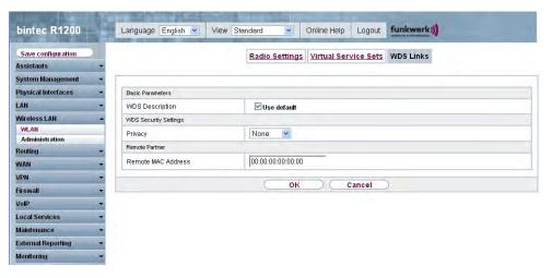
Fig. 77: Wireless LAN -> WLAN -> WDS Links -> | -> /New
