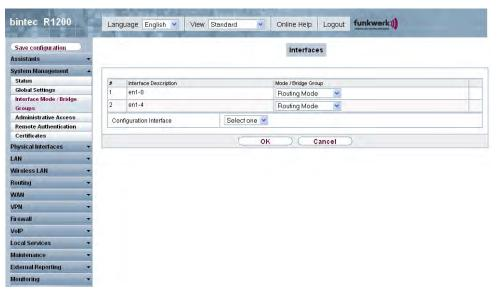
Fig. 45: System Management -> Interface Mode / Bridge Groups -> Interfaces
