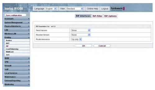
Fig. 87: Routing -> RIP -> RIP Interfaces->
