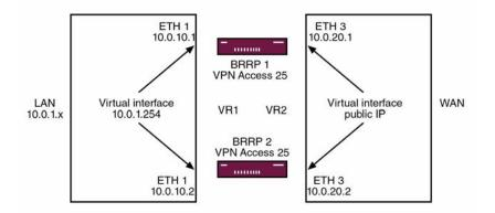
If the master gateway fails, e.g. due to a hardware fault, the backup gateway takes over the functionality of the master gateway. The backup gateway remains in hot standby mode as long as the master gateway is active. How the gateways behave in the event of a failure can be defined with a configurable set of rules.
