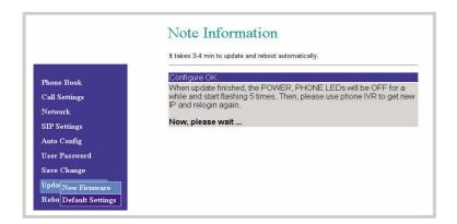
• After 3 to 4 minutes the »PHONE« LED flashes five times, thus indicating the successful completion of the firmware update. Now log back in and dial #120# to have the new IP address for the Web-based configuration identified.
