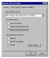
6. Click the **TCP/IP Settings...** button. Verify the IP address, name service, and compression settings are consistent with those required by the ISP and click **OK**.
