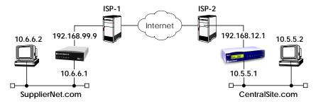
Once both BRICKs are configured for Virtual Private Networking hosts on either LAN can connect to hosts on the remote LAN. All traffic that is routed between the two networks is encrypted (user-data encryption). Individual hosts are not required to support PPP or PPTP, the VPN remains transparent.
