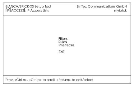
The FILTERS menu is used to configure filters. Each filter describes a subset of IP traffic and may be address, protocol, source or destination port based.
