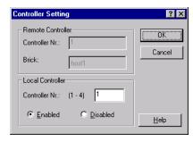
Here you can assign a different local controller number to the controller, or Enable or Disable it for CAPI connections.
