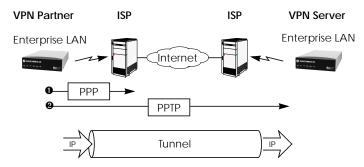
Here a Virtual Private Network that connects two enterprise LANs via the Internet is established via two VPN Servers. Either side may initiate a standard PPP link to a local ISP. Once the link is established the same server establishes a PPTP connection to the remote VPN server. Again, the ISP is unaware of its participation in the VPN.
