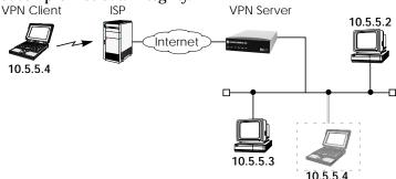
The protocol that makes VPN possible is the Point-to-Point Tunnelling Protocol or PPTP. PPTP is an IETF standard described in RFC 1171.
