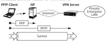
This is the most common scenario for PPTP. The remote client (mobile Win95 host) first establishes a standard PPP connection to a local ISP. The same client then initiates a second, logical connection, to the VPN Server. The ISP (and all intermediate Internet routers), unaware that it is participating in a VPN, simply routes IP packets from the PPTP Client.
