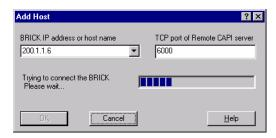
This may take a couple of seconds. If the connection fails make sure the BRICK is switched on, connected to the network, the IP address and CAPI TCP port are correct, and try again.
