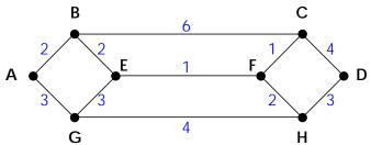
In OSPF each link has a cost associated with it (typically some fixed number divided by the bandwidth of the link). Routes are calculated and selected according to the least cost of the overall path a packet will travel. Thus in shortest-path routing the best path is also the fastest path (theoretically), regardless of the number of stations a packet travels through.
