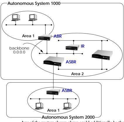
Any of the routers shown above could additionally be the Designated Router or Backup Designated Router for its respective network.
