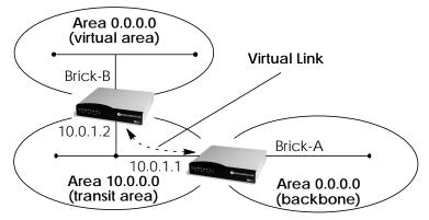
A virtual interface must be defined on each of the ABRs by creating an entry in the *ospfVirtIfTable*. This is done by setting the *ospfVirtIfNeighbor* and *ospfVirtIfAreaID* objects.
