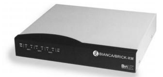
The BIANCA/BRICK-XM satisfies all the requirements of today's LAN - WAN connections by combining the functions of a Gateway, Router, Bridge, X.25 Switch and Telematic Server in a single, compact product.
