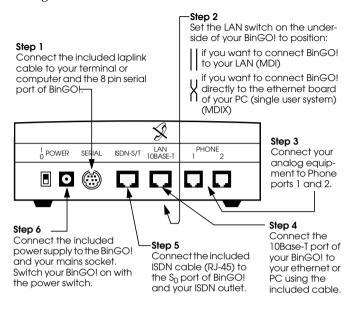
The two RJ-45 cables included with your BinGO! are identical, and can both be used for connecting BinGO! to the ISDN as well as the ethernet.
